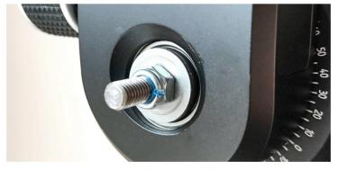
It is possible to "fine tune" the manual friction but it is not something I would rush into as I think you need time to get used to the head. This friction arrives pre-set from Cambo, presumably set up using one of their cameras and is adjusted by removing the manual locking knobs and tightening or loosening the friction setting using an 8mm spanner.
