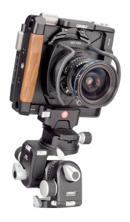
The round silver knobs are geared and adjust the tilt and pivot. These have a grip covered with a black indented material, this is quite firm and is probably a type of plastic. There are three; the two larger ones control the pivot and tilt function and the smaller one locks the QR plate in place. This is an ARCA style clamp and it works very effectively. The camera plate has two small studs front and rear that fit into two cut outs in the head
